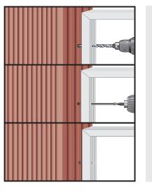
Place the window in the wall opening, adjust and drill holes. Fix the window with CELO window frame screws FBS-Z.
