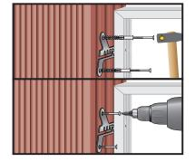
Secure ProtectFIX with two CELO multifunction frame plugs MFR SB 10-80 TX in the base material.
