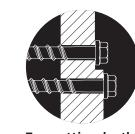
Two setting depths for a higher application flexibility (for BTS6 longer than 55 mm)
