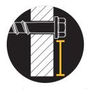
**Expansion-free anchoring** allows low edge distances and spacing
